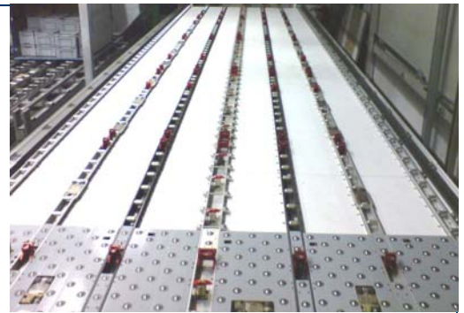
A350-900XWB FWD Cargo Compartment Mockup
