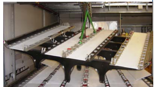
TELAIR proprietary Modular Cargo System (MODCAR) Technology using CFRP floorbeams, roller tracks and continuous side guides
