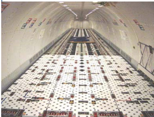
B767-300BCF main deck powered cargo system including 16ft, 20ft and 463L pallets and CMC
